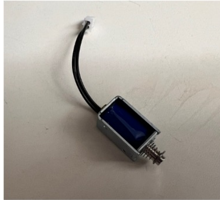
Figure 5: A solenoid, an example of a coil with a job to do (move a metal piston on the inside)
